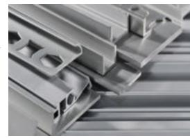
that they enhance the structural strength of the assembly. Multi-functional parts can be extruded that incorporate additional features such as wiring channels or other features for attaching body panels.
